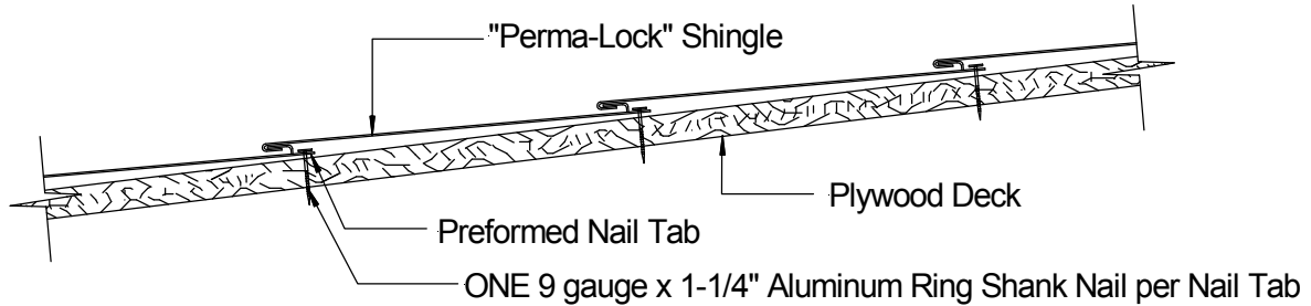
Typical Assembly - Section View
